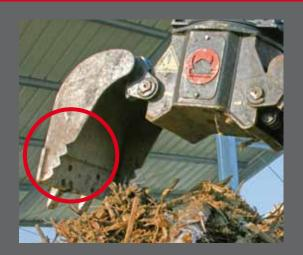
The shells are made completely of Hardox and are extremely low in wear. In order to minimize shrinkage, this grab is additionally equipped with reinforcement strips on the inside of the shells.
