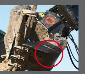
The grab's bottom is completely sealed all the way around. This protects the parts on the inside from damage due to demolition materials, such as iron, rocks, or wood.
